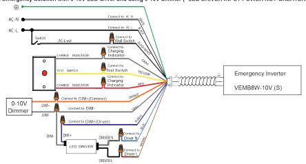
$2. \ Emergency \ Solution \ with \ 0-10V \ LED \ driver, \ without \ using \ 0-10V \ dimmer \ (^{\star} \ LED \ DRIVER \ INPUT \ POWER \ NOT \ GREATER \ THAN \ 50W)$
