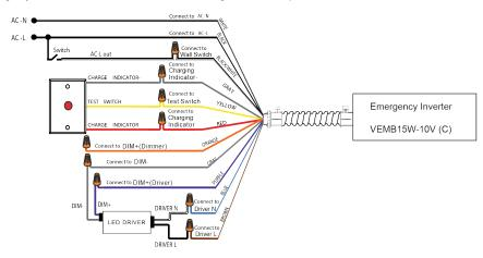
3. Emergency Solution with non-dimming LED driver (\* LED DRIVER INPUT POWER NOT GREATER THAN 15W)
