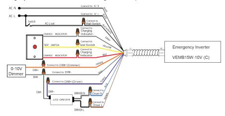
$2.\ Emergency\ Solution\ with\ 0\text{-}10V\ LED\ driver,\ without\ using\ 0\text{-}10V\ dimmer\ (*\ LED\ DRIVER\ INPUT\ POWER\ NOT\ GREATER\ THAN\ 80W)}$
